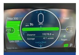
The displays in electric vehicles inform drivers of the status of the battery and estimated driving range along with other information on the car's performance.
